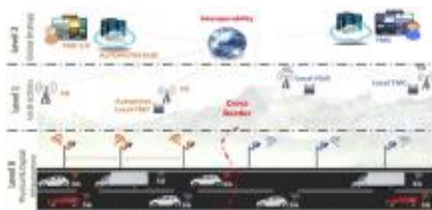
Figure 1-5: Road operator management levels
